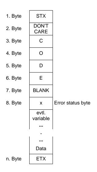
Error status byte: Value is zero: Device without error. Value is not zero: Device with one or more errors.
